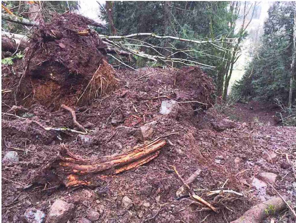
Photograph 10. – Debris lobe on 20 degree slope in partial deposition zone.
